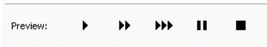
Figure 19: Buttons for play back of a sequence, play (speed x1, x10, x100), pause and stop (from left to right)
