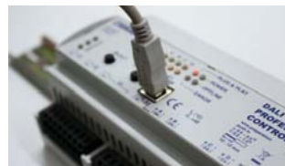
02 Commission the controller via USB connection to the PC
