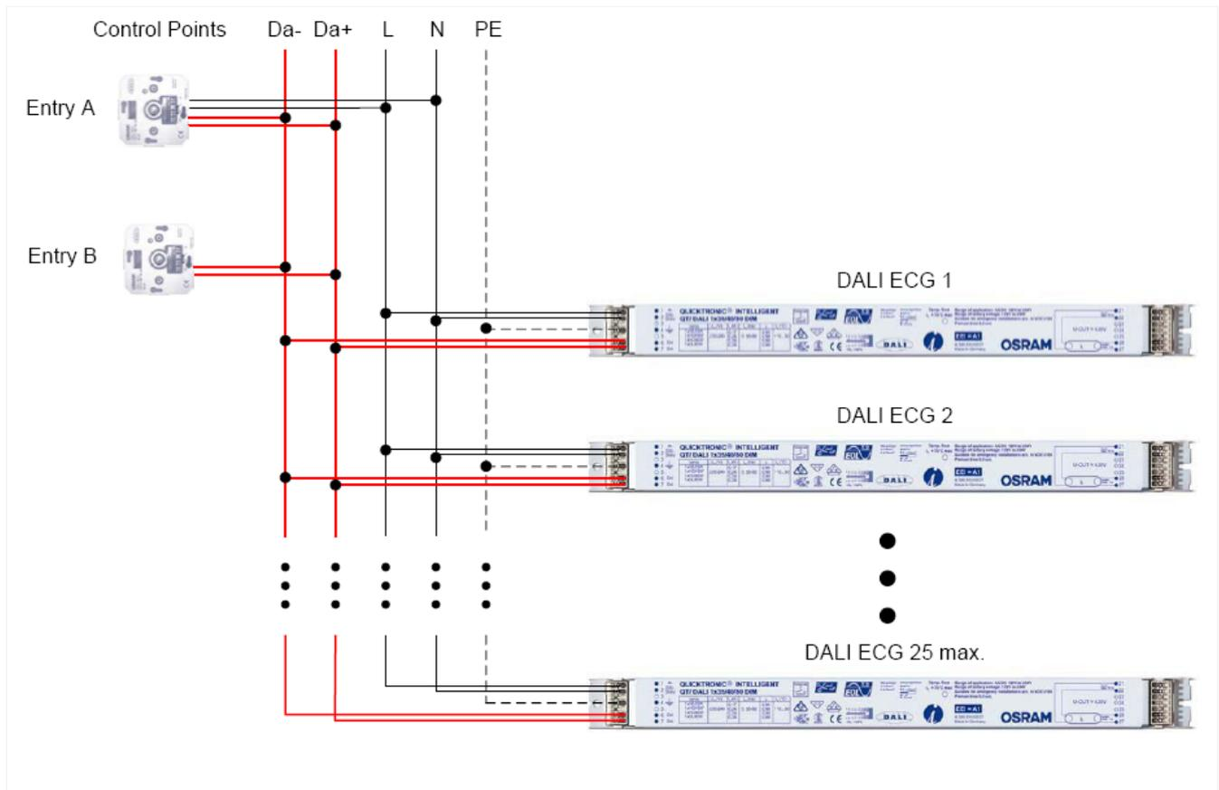
Figure 3: Wiring scheme of a conference room
