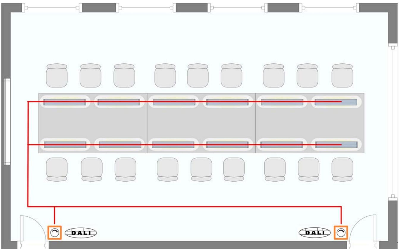
Figure 2: DALI wiring layout
