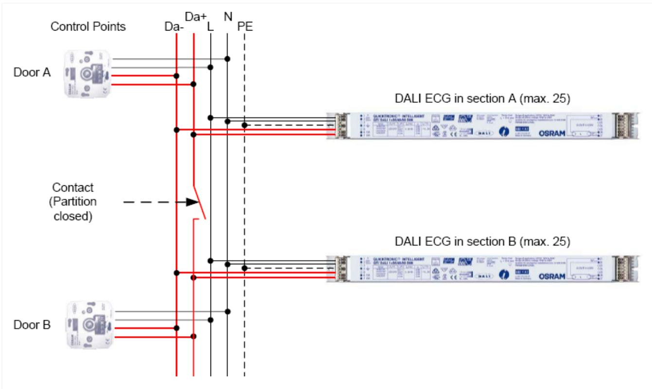
Figure 6: Wiring scheme of a room with partition
