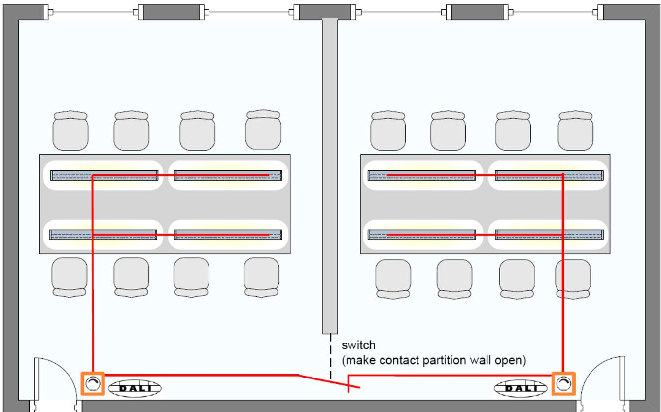
Figure 5: DALI wiring layout in a dividable room
